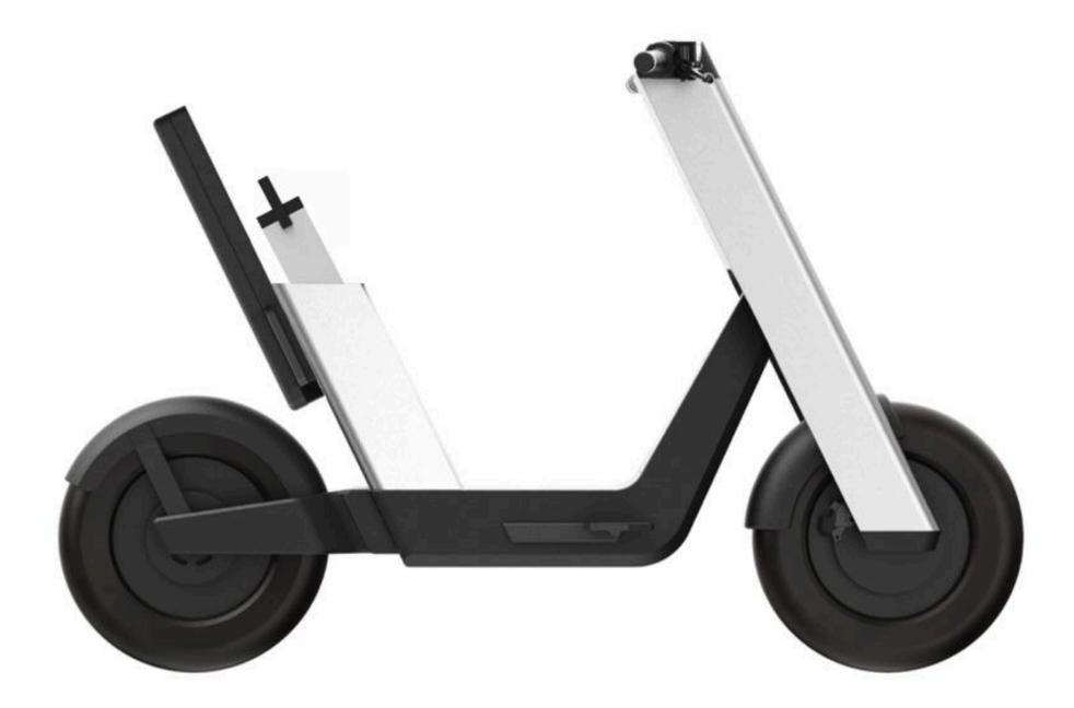
High-capacity swappable battery that can be charged indoors or directly on the vehicle.
